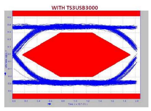
Figure 14. 480-Mbps USB 2.0 Eye Pattern for USB Switch
