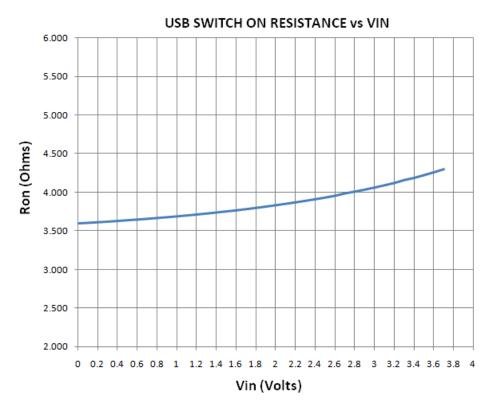
Figure 16. ON-Resistance vs. VI for USB Switch
