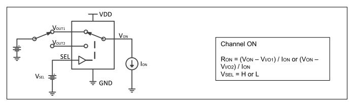
Figure 2. ON State Resistance (R<sub>ON</sub>)
