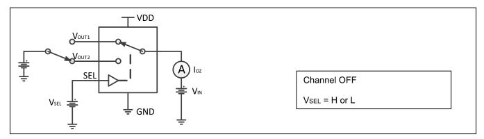
Figure 3. OFF Leakage Current (I<sub>OZ</sub>)
