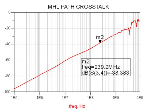
Figure 21. Cross talk vs. Frequency for MHL Path
