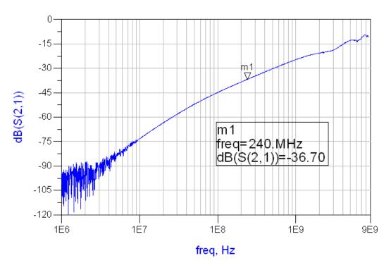
Figure 19. Off Isolation vs. Frequency for MHL Path
