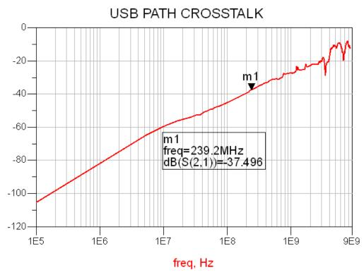
Figure 22. Cross talk vs. Frequency for USB Path
