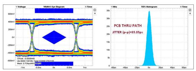
Figure 5. Eye Pattern and Time Interval Error Histogram: 0.7 Gbps With No Device
